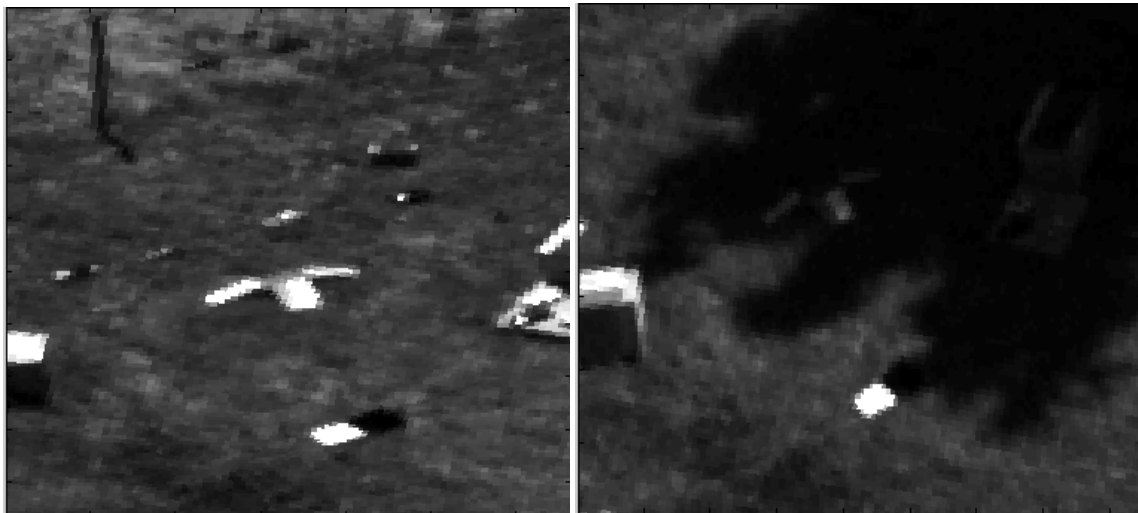
Figure 86. (Left) The green band of the cropped fused morning data subset is shown as an intensity image after converting to reflectance values. (Right) The green band of the fused afternoon data subset is shown as an intensity image after converting to reflectance values.
