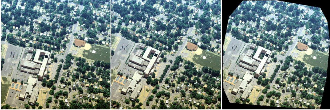
Figure 57. Several RGB DIRSIG images are displayed to illustrate the multiple sensor registration process for a solar zenith angle of 20°. (Left) The polarimetric data was drawn from an image captured at a sensor zenith angle of 30° and a sensor azimuth angle of 185°. (Center) The hyperspectral data was drawn from an image captured at a sensor zenith angle of 30° and a sensor azimuth angle of 195°. (Right) The hybrid image contains registered polarimetric and hyperspectral data from multiple sensors.
