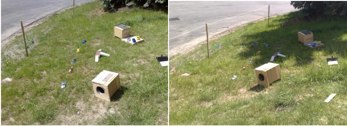
Figure 81. (Left) The morning data collect represented favorable polarimetric sensing conditions. All vehicles in the scene were sunlit. (Right) The afternoon data collect represented poor polarimetric sensing conditions. Additionally, many of the target vehicles were shadowed.
