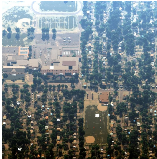
Figure 58. RGB DIRSIG image rendered with a solar zenith angle of 55^\circ , a sensor zenith angle of 40^\circ , and a sensor azimuth angle of 180^\circ .
