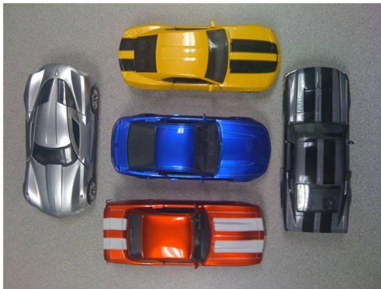
Figure 82. The vehicles staged throughout the scene were 1:32 die cast metal model cars. Reflectance measurements of the vehicles were made under direct sunlight before the imagery was collected. Next, sample sections of siding material, roofing material,
