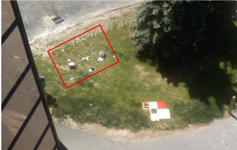
Figure 80. The ROI for the multispectral / polarimetric data fusion experiment is outlined in red. This image shows the conditions for the morning data collect, with a solar zenith angle of 26^\circ , a sensor zenith angle of 48^\circ , and a relative azimuth angle between the sensor and the sun of 160^\circ .
