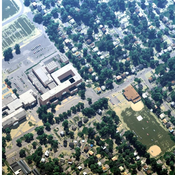
Figure 41. An RGB image of the synthetic scene was observed with a solar zenith angle of 34^\circ , a sensor zenith angle of 30^\circ and a sensor azimuth angle of 170^\circ from the sun.
