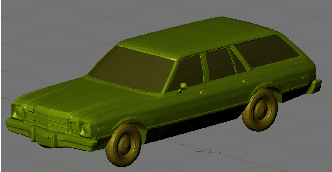
Figure 11. Subaru wagon model provided by AFOSR for use in DIRSIG. Notice the level of detail—a side mirror, front grille and even door handles have been incorporated.
