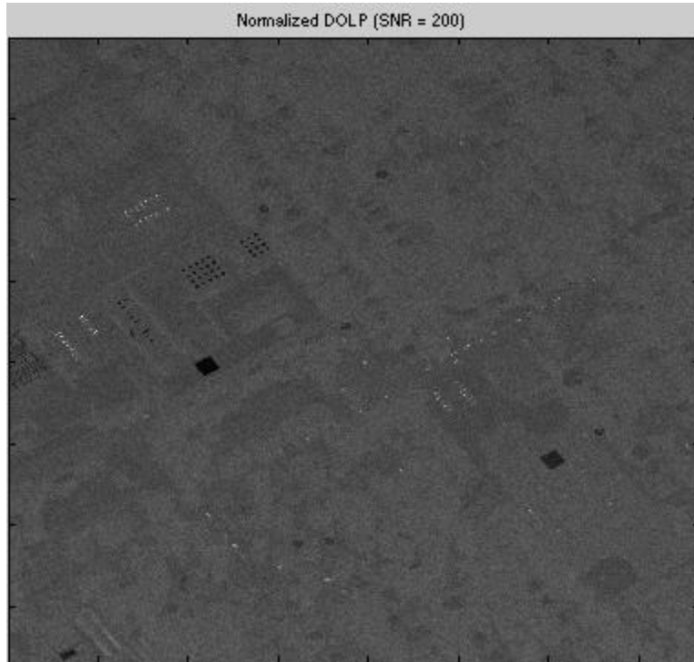
Figure 45. The polarimetric information from the scene was incorporated as DOLP values in an additional band for the SPOT algorithm.
